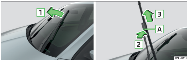
Fig. 288 Changing the front windscreen wiper blade
