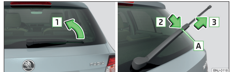
Fig. 289 Changing the rear window wiper blade
