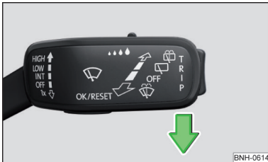
Fig. 287 Setting the service position for the wiper arms
