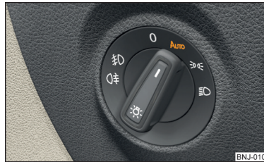
Fig. 56 Light switch: Position AUTO
