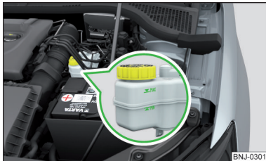
Fig. 262 Brake fluid reservoir
