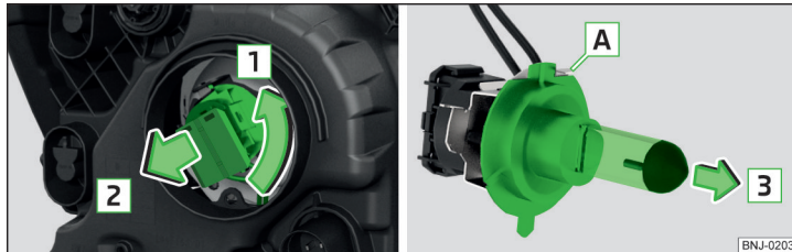
Fig. 303 Changing the bulb for the main beam
