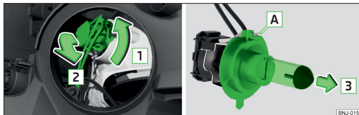
Fig. 302 Changing the bulb for the low beam
