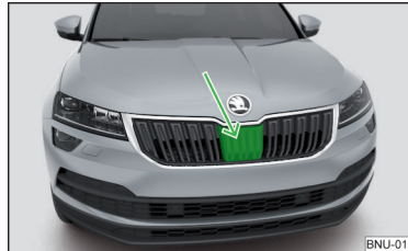
Fig. 257 Installation location of the radar sensor
