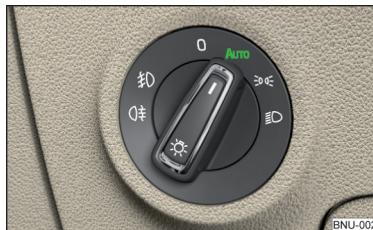
Fig. 64 Light switch: Position AUTO
