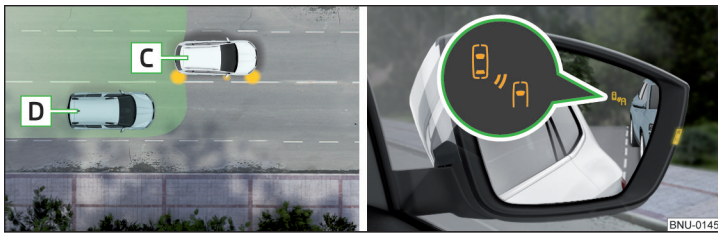
Fig. 269 Driving situation / indicator light in the right outside mirror indicates the driving situation
