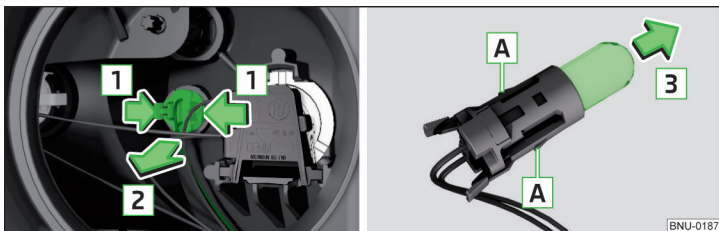
Fig. 348 Change the light bulb for the parking light
