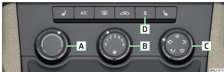
Fig. 157 Controls of the heating / air conditioning
