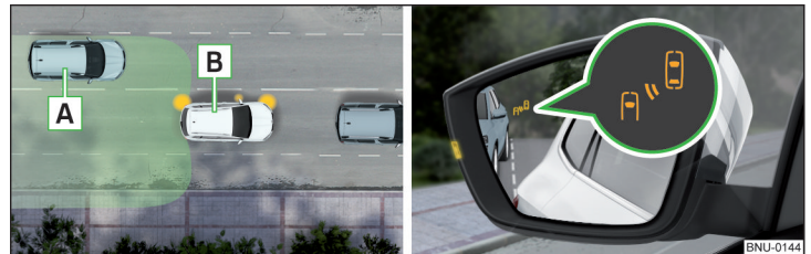
Fig. 268 Driving situation / indicator light in the left outside mirror indicates the driving situation
