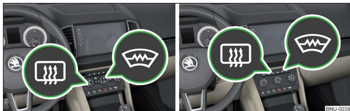
Fig. 73 Buttons for the front and rear window heater: Climatronic / manual air conditioning
