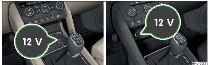
Fig. 126 Cover of the 12 volt power outlet
