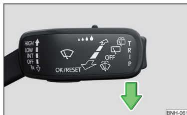
Fig. 337 Setting the service position for the wiper arms
