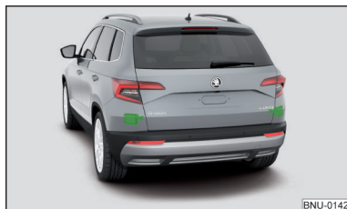
Fig. 266 Installation location of the radar sensors
