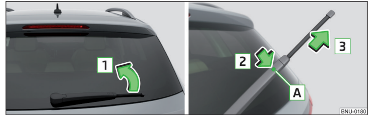
Fig. 339 Replace the rear window wiper blade
