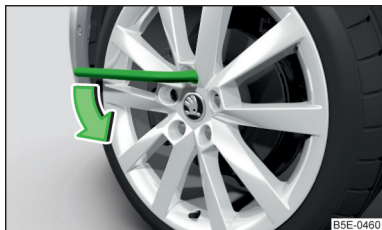
Fig. 322 Loosening the wheel bolts
