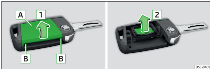
Fig. 330 Open the cover/remove the battery
