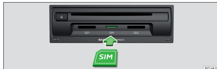
Fig. 198 Insert SIM card in the external module
