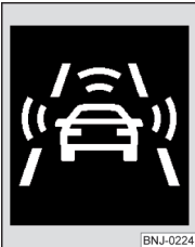
Fig. 289 Instrument cluster display: Advance warning or emergency braking at low speed
