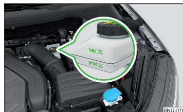
Fig. 310 Brake fluid reservoir
