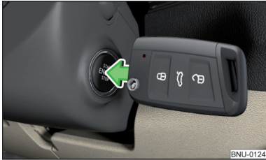
Fig. 245 Engine start - hold key on button
