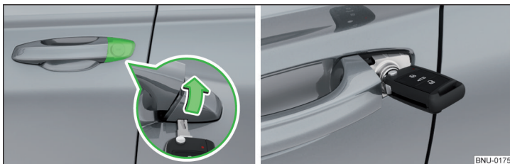
Fig. 333 Handle on the driver's door: Open lock cover / lock cylinder with key
