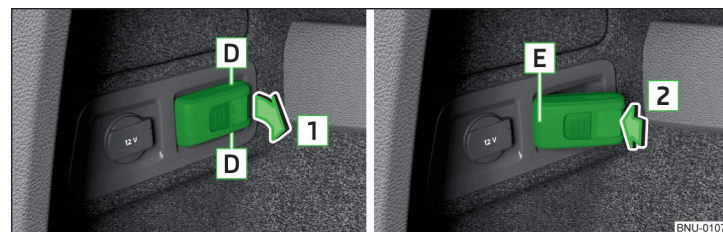
Fig. 154 Removing light/inserting light
