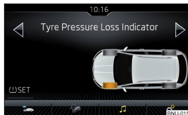
Fig. 296 Button for storage / screen display example: a tyre pressure change at the front left is shown
