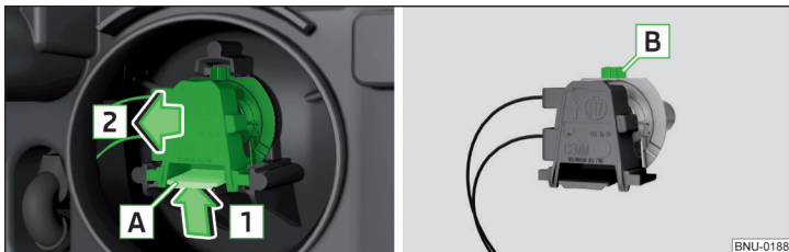
Fig. 347 Removing bulbs for low and main beam
