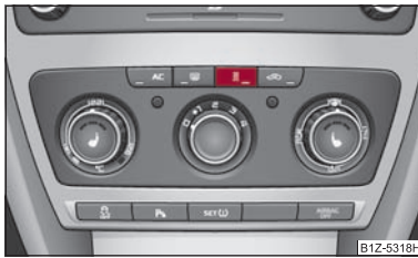
Fig. 109 Button for direct switching on/off of the auxiliary heating (auxiliary heating and ventilation) on the operating part of the air conditioning system
