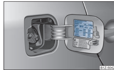
Fig. 170 An opened fuel filler flap with a tyre size and tyre inflation pressure table
