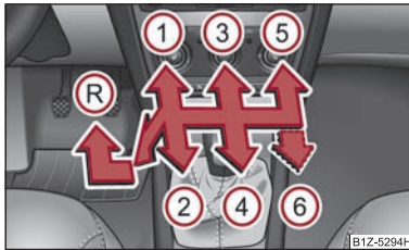
Fig. 113 The shift pattern: 5-speed or 6-speed manual gearbox
