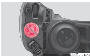
Fig. 194 Removing the light bulb for the turn signal light
