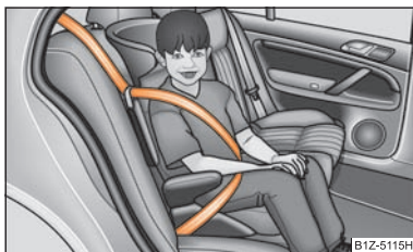
Fig. 147 Child seat in Group 2 installed on the rear seat facing the direction of travel
