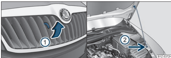
Fig. 162 Radiator grille: Locking lever/securing the bonnet with the bonnet support
