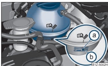
Fig. 165 Engine compartment: Coolant expansion bottle
