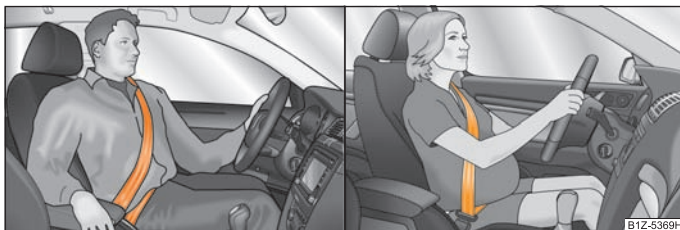
Fig. 132 Routing of belt webbing over the shoulders and the lap belt/Routing of belt webbing for an expectant mother
