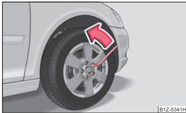
Fig. 179 Changing a wheel: Slackening wheel bolts
