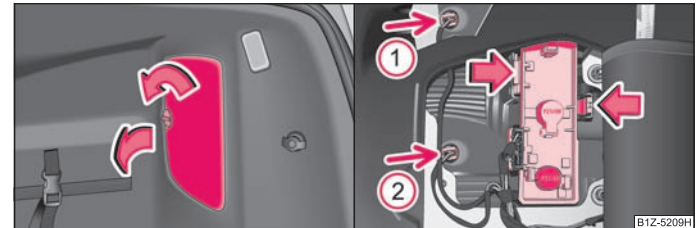
Fig. 201 Luggage compartment: Cover for the lamp holder/removing the lamp holder
