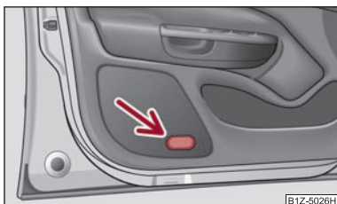
Fig. 46 Front door: Warning light
