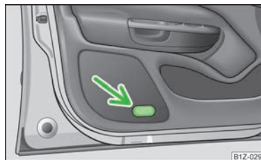
Fig. 31 Front door: Warning light
