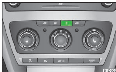
Fig. 91 Button for direct switching on/off of the auxiliary heating (auxiliary heating and ventilation) on the operating part of the air conditioning system
