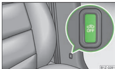
Fig. 14 Button for interior monitor and towing protection monitoring
