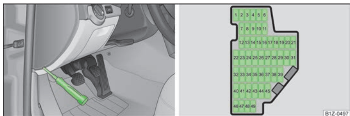
Fig. 158 Fuse box cover in the dash panel/schematic diagram of the fuse box
