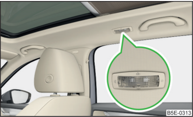
Fig. 56 Interior lights at the rear: Variant 3
