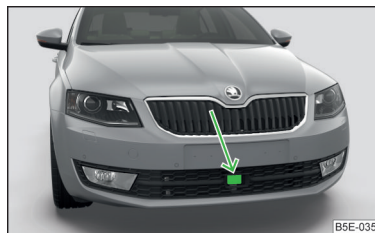
Fig. 150 Mounting location of the radar sensor
