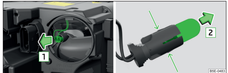
Fig. 239 Headlights with Xenon light: Bulb for additional parking light
