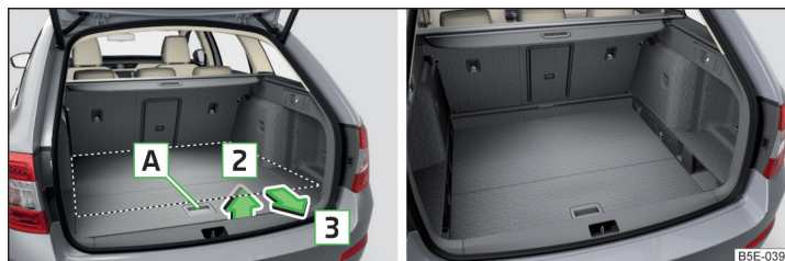
Fig. 119 Set variable loading floor to the lower position / variable loading floor in the lower position
