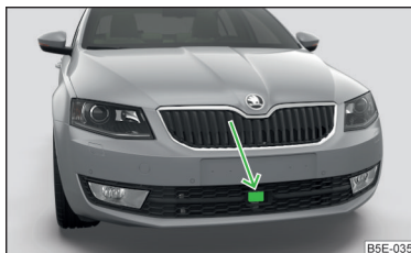
Fig. 160 Mounting location of the radar sensor
