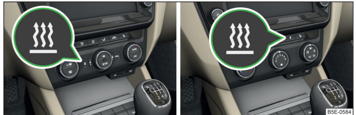
Fig. 132 Button for direct power on / off of the auxiliary heating (heating and ventilation) on the front panel of the Climatronic / manual air conditioning
