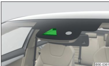
Fig. 174 Camera viewing range for traffic sign recognition
