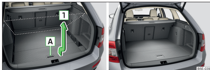
Fig. 118 Set variable loading floor to the upper position / variable loading floor in the upper position
