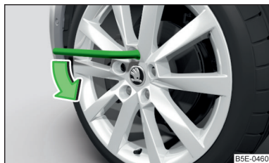
Fig. 213 Changing a wheel: Loosening the wheel bolts
