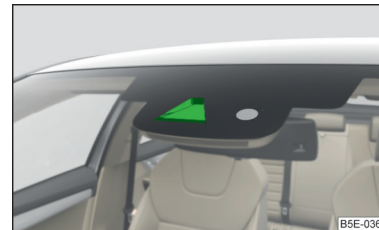
Fig. 171 Camera viewing window for Lane Assist
