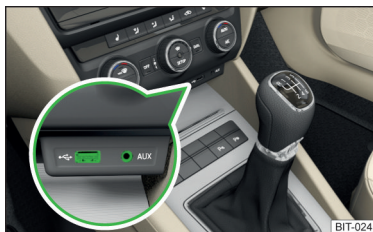
Fig. 101 Installation locations of the AUX and USB inputs
