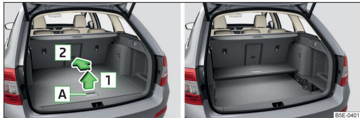
Fig. 120 Fold up variable loading floor / folded variable cargo floor in the upper position
