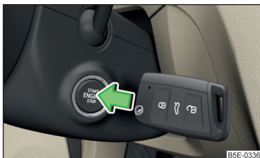
Fig. 136 Starting the engine - press the button with the key
