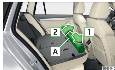
Fig. 124 Removing the net partition housing
