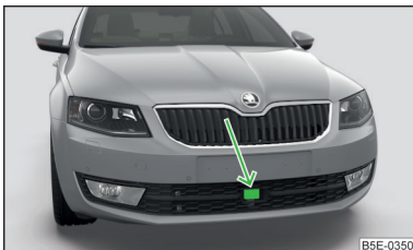
Fig. 166 Mounting location of the radar sensor
