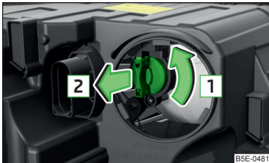
Fig. 238 Bulbs for main beam, daytime running lights, and parking light
