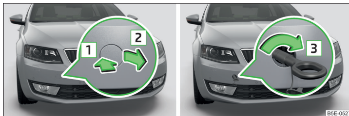
Fig. 220 Removing the cap / installing the towing eye
