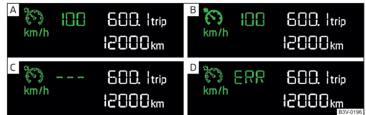
Fig. 158 Segment display: Examples of status displays the CCS
