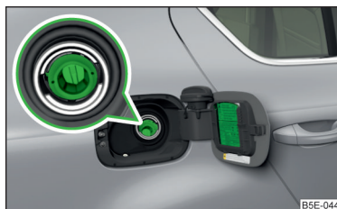
Fig. 193 Fuel filler tube on vehicles with diesel engines
