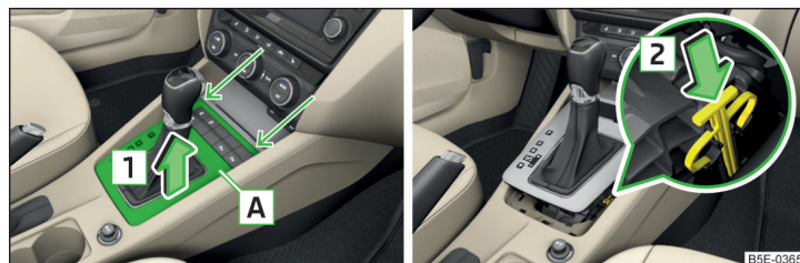
Fig. 228 Selector lever-emergency unlocking
