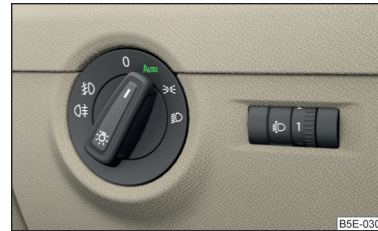
Fig. 54 Light switch: AUTO position
