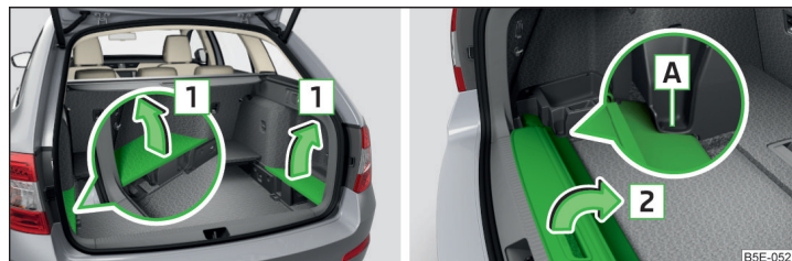
Fig. 113 Remove the side panels of the luggage compartment/stow the roll-up luggage compartment cover
