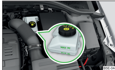
Fig. 201 Brake fluid reservoir
