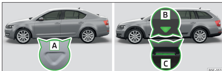
Fig. 214 Jacking points for the jack Version 1 / version 2
