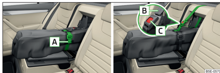
Fig. 113 Tighten ribbon / secure through-loading bag
