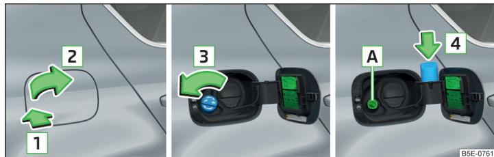
Fig. 313 Open fuel filler flap / unscrew tank cap / place the tank cap on the fuel filler flap
