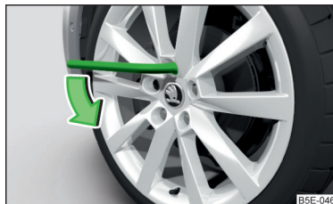
Fig. 330 Loosening the wheel bolts
