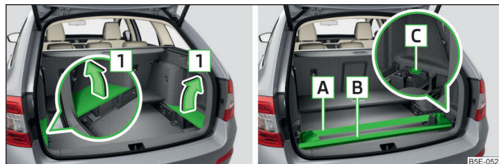
Fig. 150 Remove the side panels of the luggage compartment/stow the roof rack
