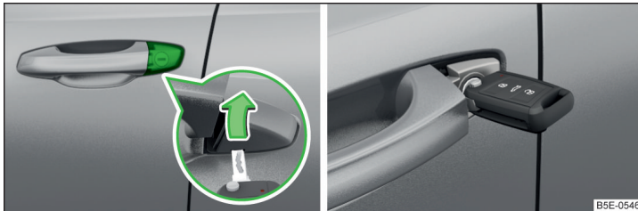
Fig. 342 Handle on the driver's door: Open lock cover / lock cylinder with key
