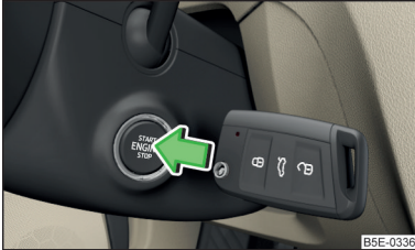
Fig. 239 Starting the engine - press the button with the key
