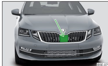
Fig. 249 Installation location of the radar sensor
