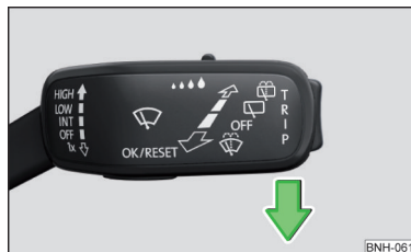
Fig. 346 Setting the service position for the wiper arms
