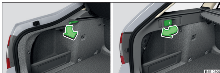
Fig. 87 Fold the backrest forward from the luggage compartment: Version 1/version 2
