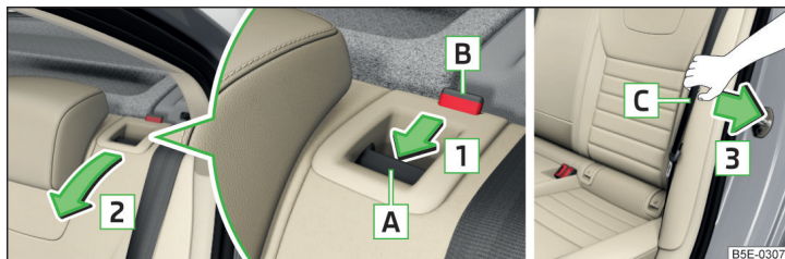
Fig. 86 Fold the seat backrest forwards from the interior/pull the belt for the side trim
