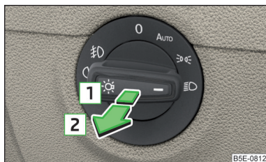
Fig. 68 Light switch – switch on front and rear fog lights
