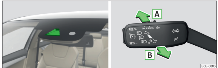
Fig. 67 Installation location of the sensor / system on/off
