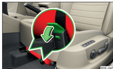
Fig. 325 Release the fire extinguisher
