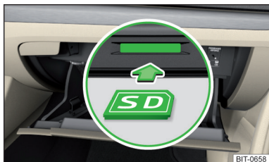
Fig. 183 Columbus, Amundsen, Bolero: Insert the SD card
