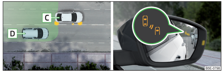
Fig. 260 Driving situation / indicator light in the right outside mirror indicates the driving situation
