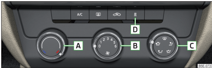
Fig. 151 Controls of the heating / air conditioning
