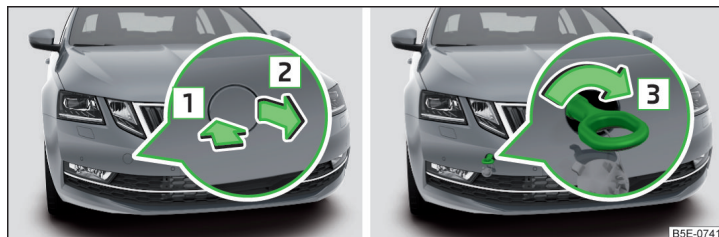
Fig. 336 Remove cap / install towing eye
