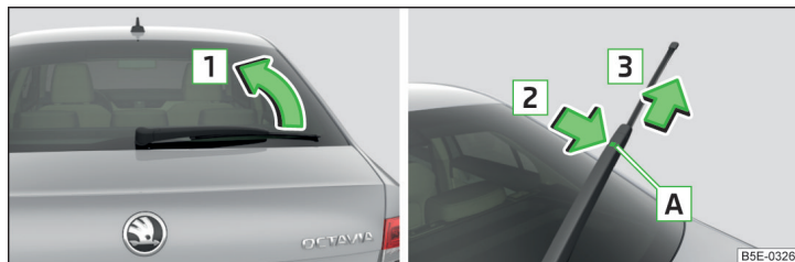
Fig. 348 Replace the rear window wiper blade
