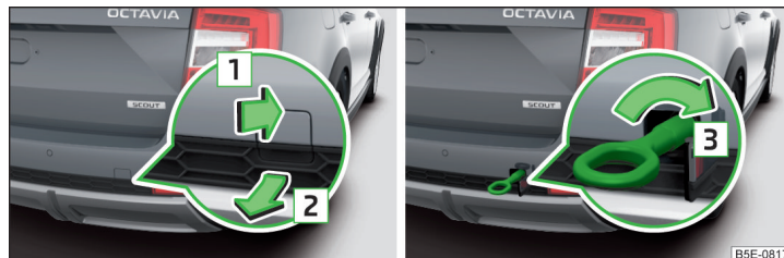
Fig. 338 Remove cap / install towing eye - Variant 2
