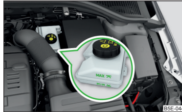
Fig. 319 Brake fluid reservoir
