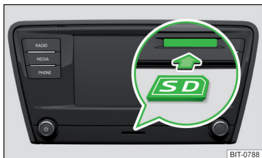
Fig. 184 Swing: Insert the SD card
