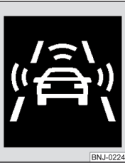
Fig. 286 Display in the instrument cluster: Advance warning or emergency braking at low speed
