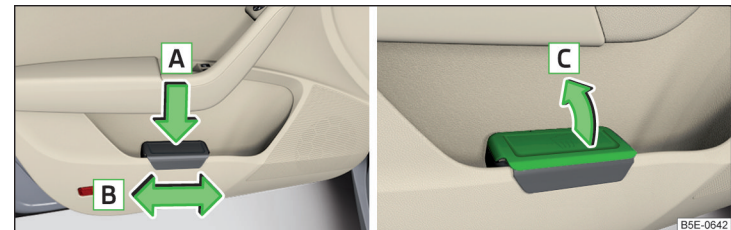
Fig. 101 Waste container: inserting and moving/opening
