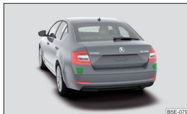
Fig. 257 Installation location of the radar sensors
