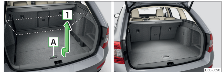
Fig. 142 Set variable loading floor to the upper position / variable loading floor in the upper position
