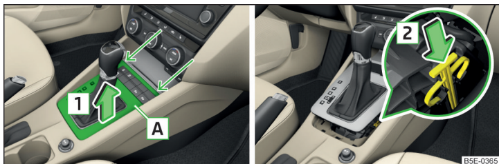
Fig. 345 Remove the cover/release the selector lever
