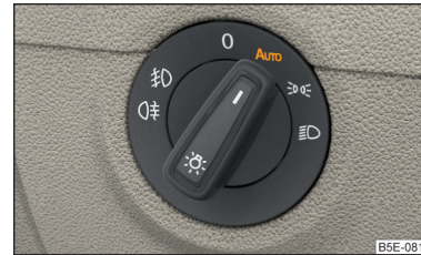
Fig. 66 Light switch: Position AUTO
