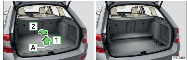
Fig. 144 Fold up variable loading floor / folded variable cargo floor in the upper position
