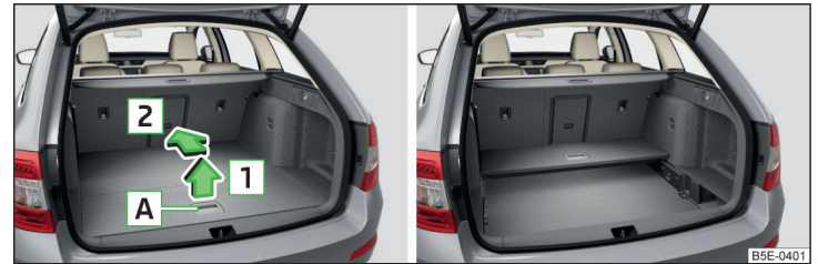
Fig. 145 Fold up variable loading floor / folded variable cargo floor in the upper position
