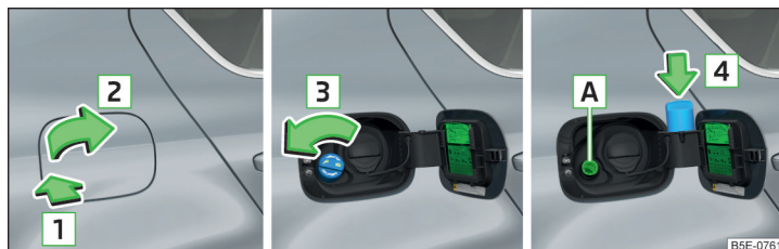
Fig. 314 Open fuel filler flap / unscrew tank cap / place the tank cap on the fuel filler flap
