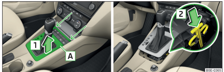
Fig. 345 Remove the cover/release the selector lever
