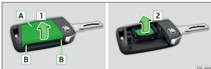
Fig. 340 Open the cover/remove the battery
