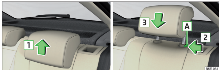
Fig. 93 Setting the height of the back headrest
