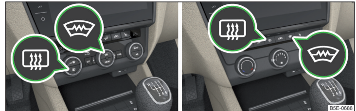
Fig. 77 Buttons for the front and rear window heater: Climatic / manual air conditioning
