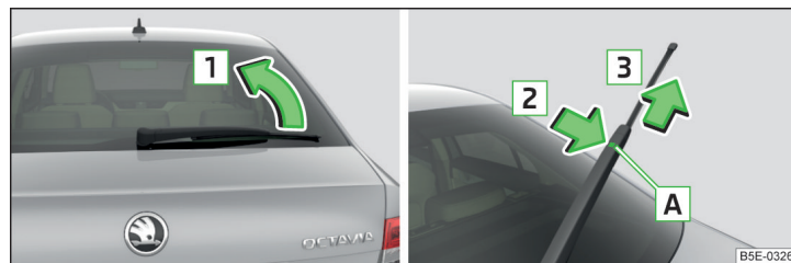
Fig. 348 Replace the rear window wiper blade
