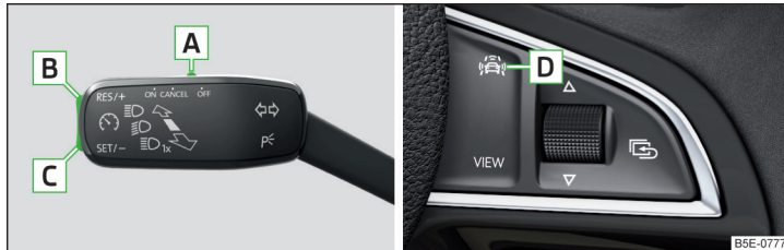
Fig. 279 Operating elements of the speed limiter: Lever / multifunction steering wheel
