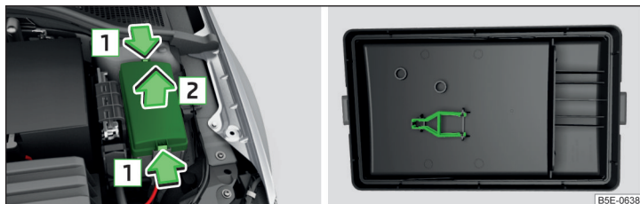
Fig. 353 Fuse box cover: Removing the cover / Plastic clip for fuses
