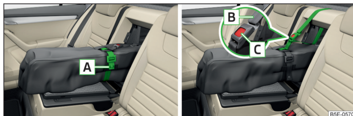
Fig. 116 Tighten ribbon / secure through-loading bag
