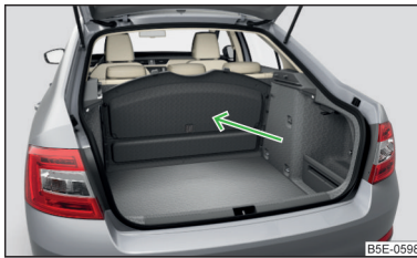
Fig. 136 Luggage compartment cover stowed behind the rear seats
