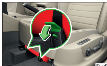
Fig. 326 Release the fire extinguisher
