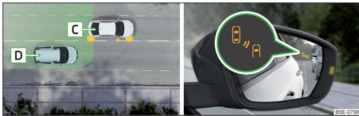
Fig. 261 Driving situation / indicator light in the right outside mirror indicates the driving situation
