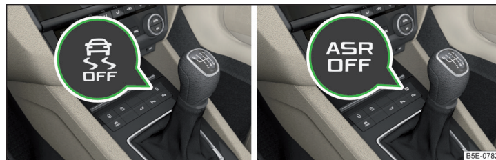
Fig. 251 System button: Vehicle with ESC / vehicle without ESC
