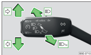
Fig. 68 Operating lever: Turn signal and main beam operation
