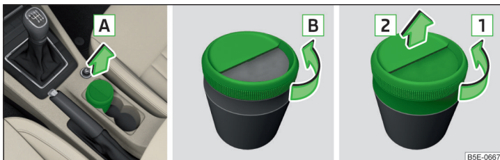
Fig. 119 Remove / open / disassemble ashtray
