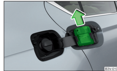
Fig. 308 Installation location of the ice scraper, removing the scraper
