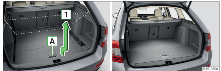
Fig. 143 Set variable loading floor to the upper position / variable loading floor in the upper position
