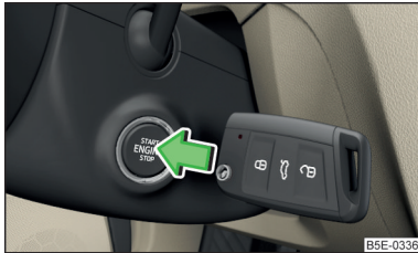
Fig. 240 Starting the engine - press the button with the key
