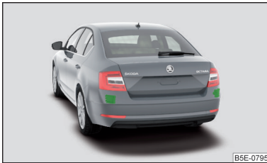
Fig. 258 Installation location of the radar sensors
