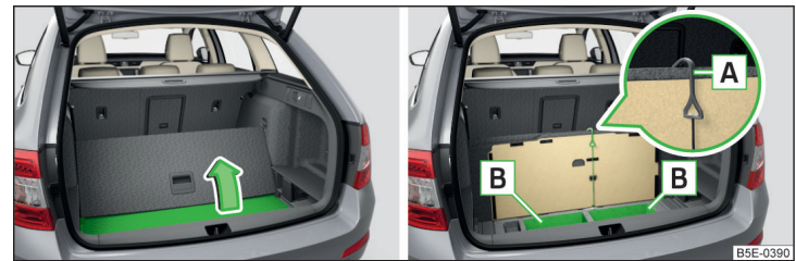
Fig. 141 Lift floor covering/storage compartments under the floor covering
