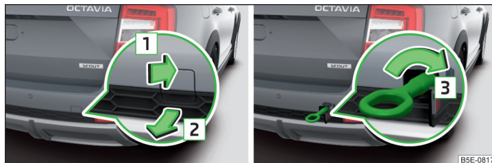
Fig. 339 Remove cap / install towing eye - Variant 2
