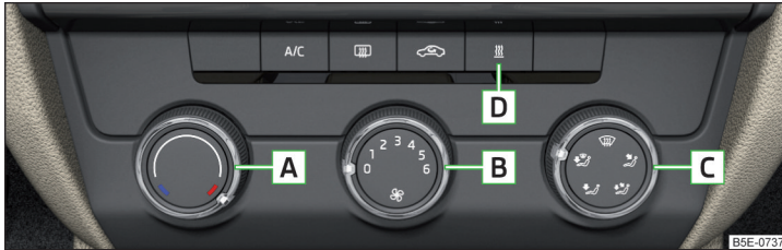
Fig. 152 Controls of the heating / air conditioning
