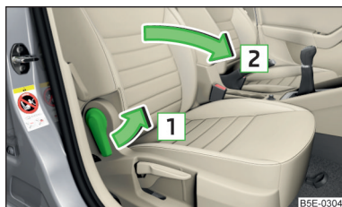
Fig. 87 Folding the front passenger seat forward
