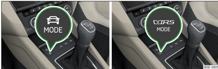
Fig. 288 Button for selecting the driving mode: Version 1/version 2
