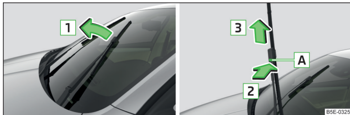
Fig. 347 Replace windscreen wiper blade
