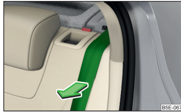
Fig. 20 Unlock the belt retractor
