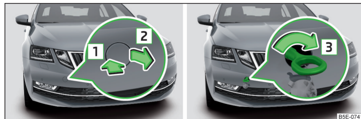
Fig. 337 Remove cap / install towing eye
