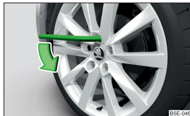
Fig. 331 Loosening the wheel bolts
