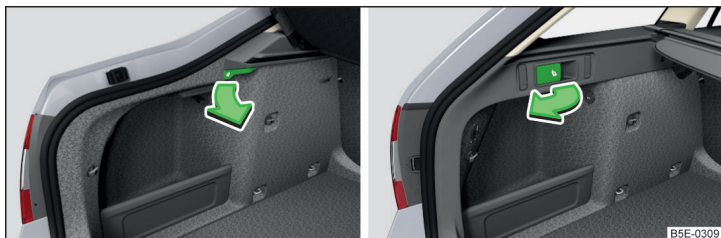
Fig. 90 Fold the backrest forward from the luggage compartment: Version 1/version 2
