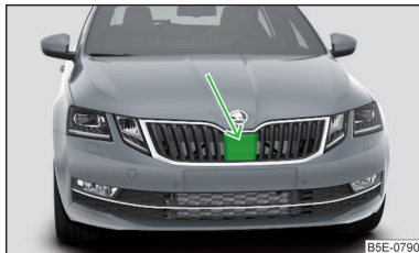
Fig. 250 Installation location of the radar sensor
