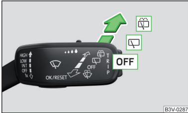
Fig. 81 Operating the windscreen wipers and washing system
