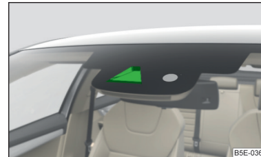
Fig. 293 Sensor for traffic sign recognition
