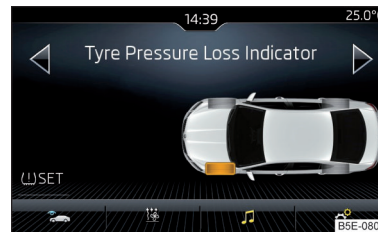
Fig. 295 Button for storage / screen display example: a tire pressure change at the front left is shown
