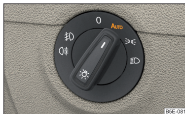
Fig. 69 Light switch: Position AUTO
