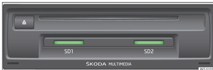
Fig. 22 SD memory card slots
