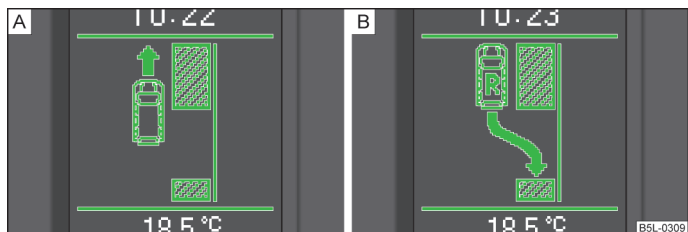
Fig. 122 Information display: Parking space detected including the information to continue driving A and to engage reverse gear B
