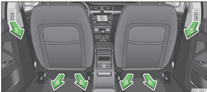
Fig. 107 Air vents at the rear
