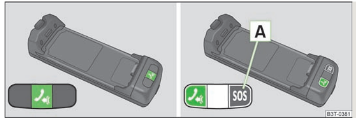
Fig. 131 Principle sketch: single-button adapter/two-button adapter
