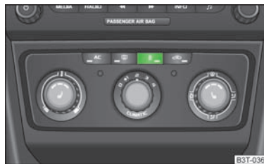
Fig. 110 Button for direct switching on/off of the auxiliary heating (auxiliary heating and ventilation) on the operating part of the air-conditioning system
