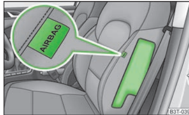
Fig. 145 Installation position of side airbag in driver seat
