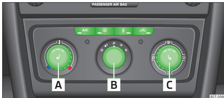
Fig. 124 The air conditioning system: Control elements
