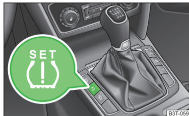
Fig. 170 Button for setting the tyre inflation pressure control value
