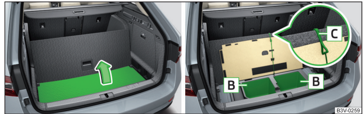
Fig. 132 Variant 2: lifting flooring & storage compartments
