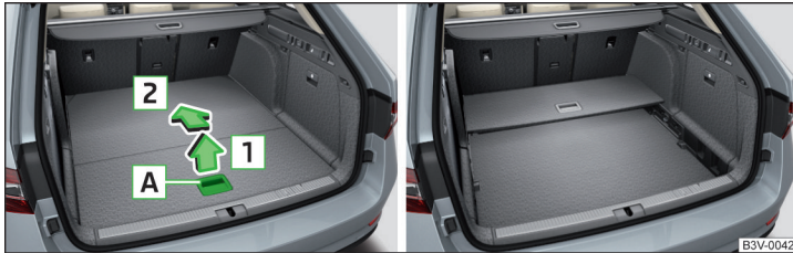
Fig. 137 Fold up variable loading floor / folded variable cargo floor in the upper position
