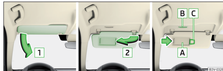
Fig. 56 Fold down flap / flip up flap / make-up mirror and parking permit holder
