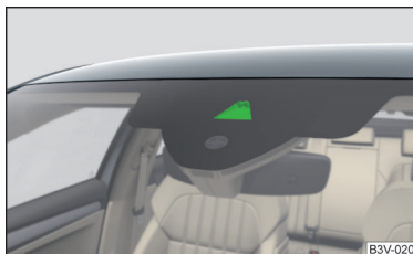
Fig. 50 Sensor window for the headlight assistant
