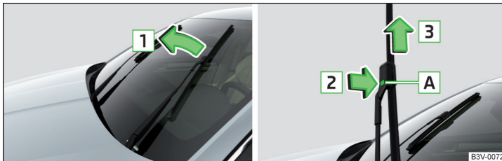
Fig. 252 Replace windscreen wiper blade
