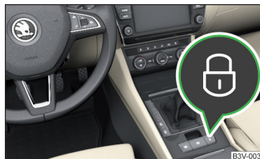
Fig. 33 Central locking button
