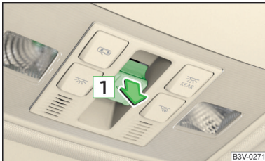
Fig. 42 Operation of the sliding/tilting roof
