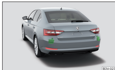
Fig. 170 Installation location of the radar sensors
