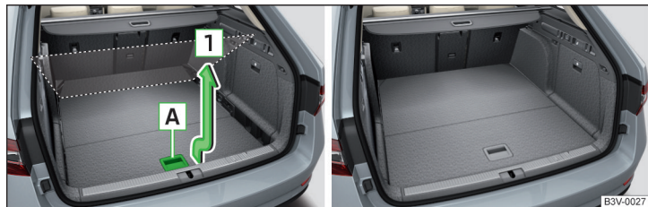
Fig. 135 Set variable loading floor to the upper position / variable loading floor in the upper position
