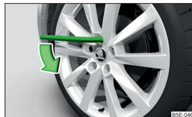
Fig. 233 Loosening the wheel bolts
