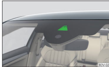
Fig. 201 Sensor for Lane Assist
