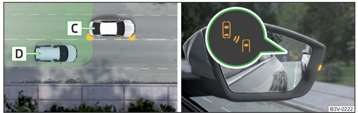
Fig. 173 Driving situation / indicator light in the right outside mirror indicates the driving situation
