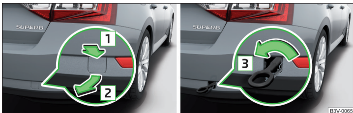
Fig. 240 Remove cap / install towing eye
