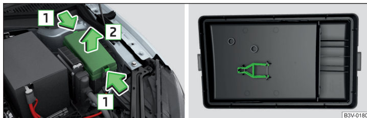
Fig. 259 Fuse box cover: removing cover / plastic clip for fuses
