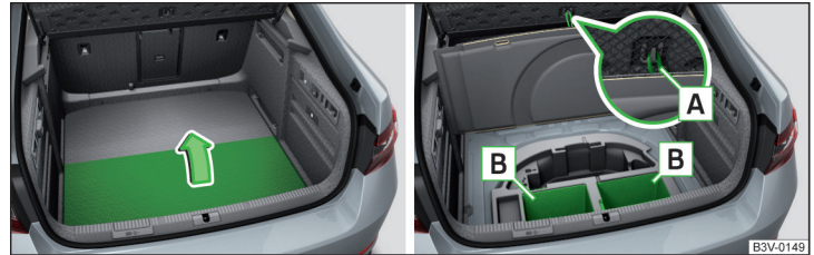
Fig. 131 Variant 1: lifting flooring & storage compartments
