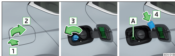
Fig. 215 Open fuel filler flap / unscrew tank cap / place the tank cap on the fuel filler flap
