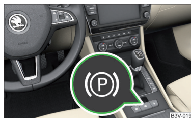
Fig. 154 Parking brake button
