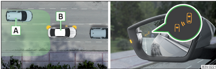
Fig. 172 Driving situation / indicator light in the left outside mirror indicates the driving situation
