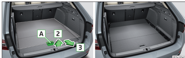
Fig. 136 Set variable loading floor to the lower position / variable loading floor in the lower position
