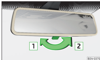
Fig. 61 Rear-view mirrors with manual dimming
