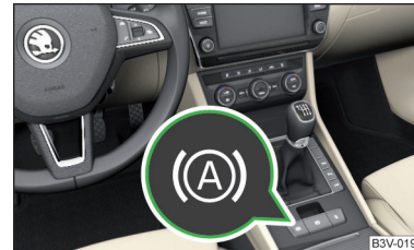
Fig. 156 The Auto-Hold function button
