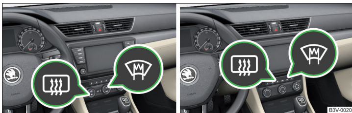
Fig. 55 Buttons for the front and rear window heater: Climatronic / manual air conditioning
