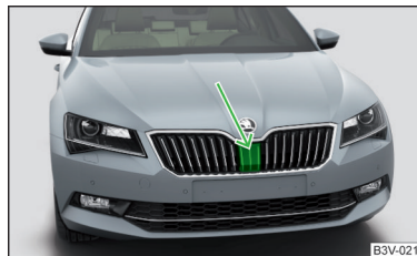
Fig. 163 Installation location of the radar sensor
