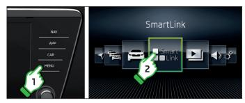
SmartLink+ allows you to display and operate certified applications of an external device connected by USB on the Infotainment screen.
