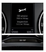
Release the button, the remaining kilometres or miles and days are shown on the display until the next service interval for 4 s
