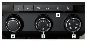
Individual functions can be adjusted or turned on by turning the knob or pressing the appropriate button. When the function is turned on, the indicator light will illuminate underneath the button.
