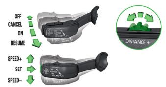
The Adaptive Cruise Control controls the set speed and the distance to the vehicle ahead without the accelerator or brake pedal being pressed.
