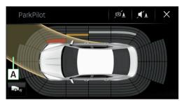
The system draws attention to obstacles in the vicinity of the vehicle via audible signals and coloured labels in the Infotainment screen.
