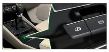
The Auto Hold function stops the vehicle rolling away during start up. The safety of the system is displayed by the warning light p lighting up in the instrument cluster.
