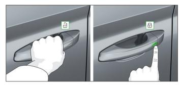
The KESSY system uses enables the vehicle to be unlocked and locked without actively using the key, using sensors in the two front door handles.
