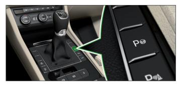
Park Assist helps drivers park in suitable parallel and perpendicular parking places or also to manoeuvre out of parallel parking spaces.
