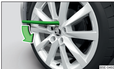
Fig. 332 Loosening the wheel bolts
