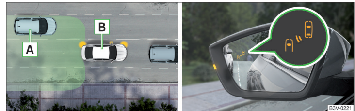
Fig. 275 Driving situation / indicator light in the left outside mirror indicates the driving situation
