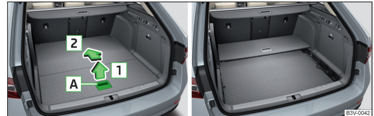
Fig. 159 Fold up variable loading floor / folded variable cargo floor in the upper position
