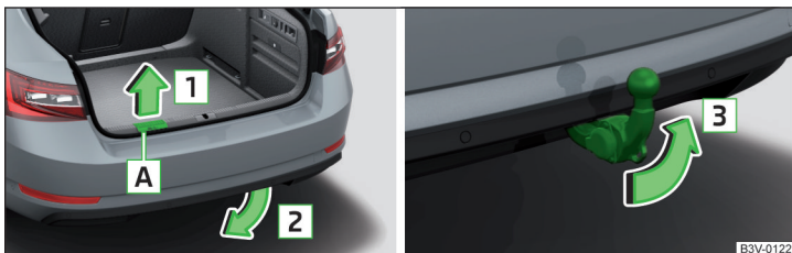
Fig. 308 Ball rod: Swivel out/in
