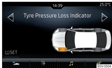
Fig. 307 Button for storage / screen display example: a tyre pressure change at the front left is shown
