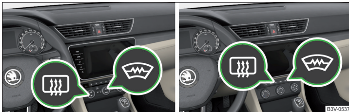
Fig. 75 Buttons for the front and rear window heater: Climatronic / manual air conditioning
