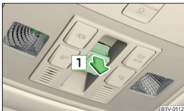
Fig. 61 Operation of the sliding/tilting roof
