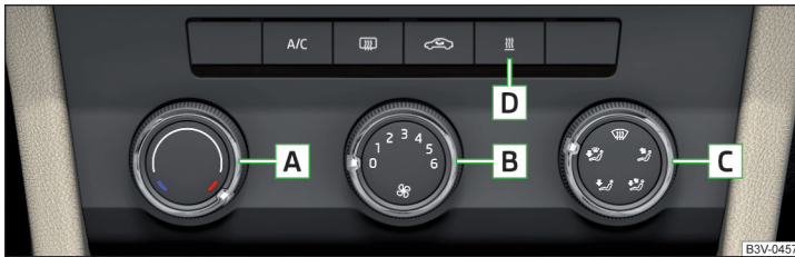
Fig. 165 Controls of the heating / air conditioning
