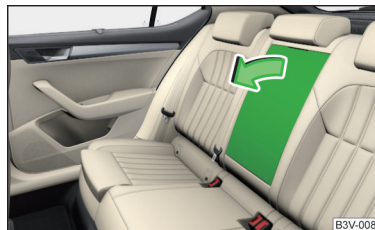
Fig. 93 Fold down armrest
