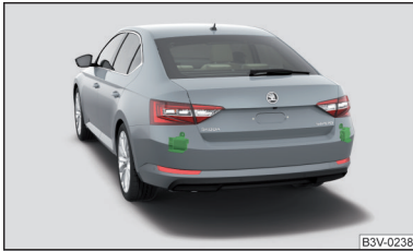
Fig. 273 Installation location of the radar sensors
