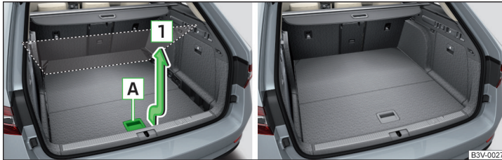
Fig. 157 Set variable loading floor to the upper position / variable loading floor in the upper position
