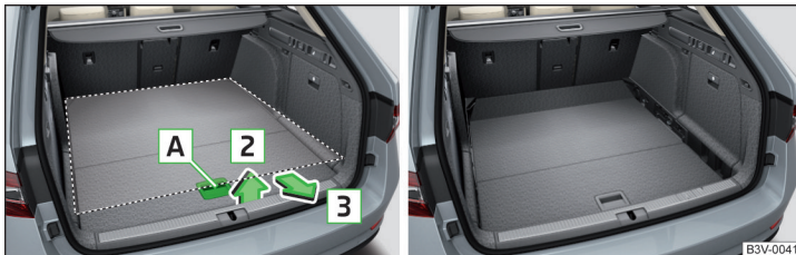
Fig. 158 Set variable loading floor to the lower position / variable loading floor in the lower position
