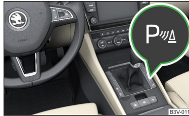
Fig. 185 Button for activation / deactivation
