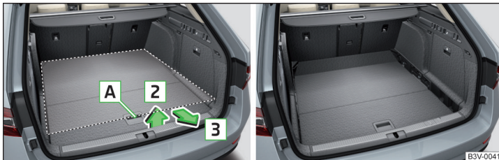
Fig. 146 Set variable loading floor to the lower position / variable loading floor in the lower position
