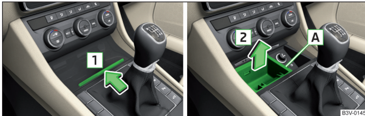
Fig. 119 Front centre console: Open storage compartment / removing ashtray
