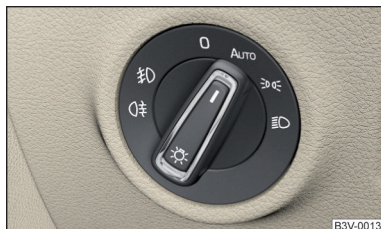
Fig. 56 Light switch: AUTO position
