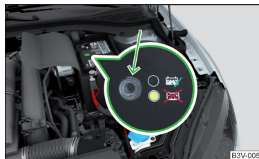
Fig. 234 Vehicle battery: Electrolyte level indicator
