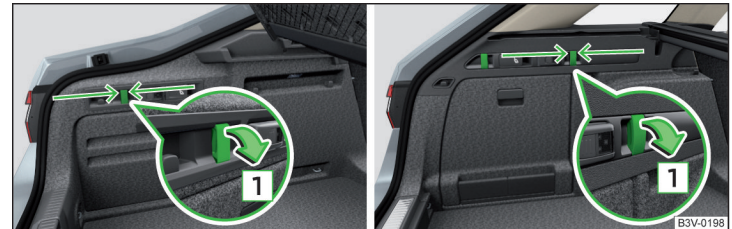
Fig. 129 Fold-down hooks: variant 1 / variant 2
