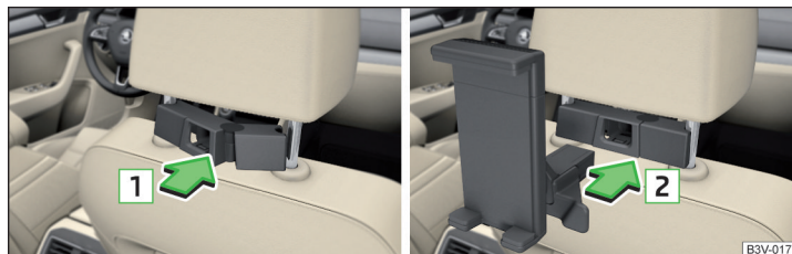
Fig. 122 Positioning the adapter/installing the holder
