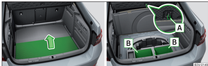
Fig. 141 Variant 1: Lifting the floor covering / Storage compartments
