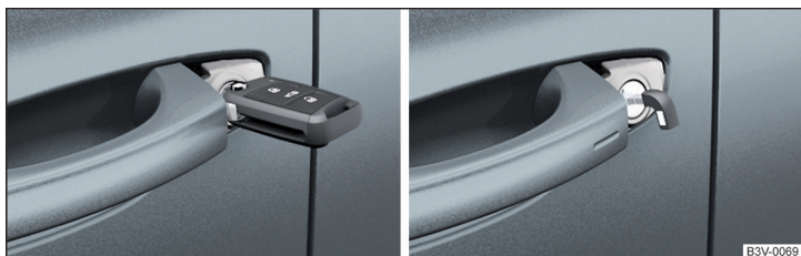
Fig. 260 Handle on the driver's door: Key / KESY
