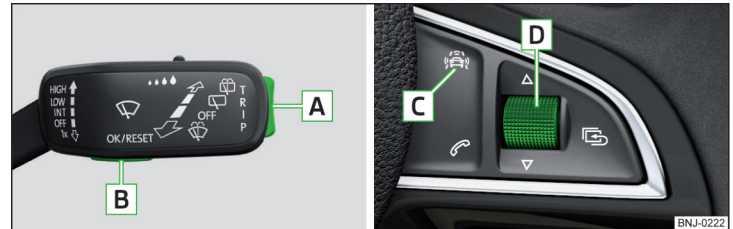
Fig. 209 Buttons/dial: on the control lever / multifunction steering wheel
