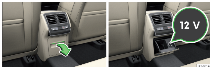
Fig. 114 Open storage compartment / cover of the 12 volt power outlet
