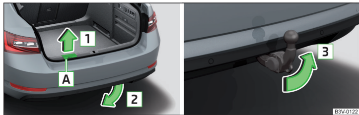
Fig. 220 Tow bar: swing in and out
