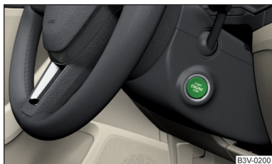
Fig. 162 Starter button (START ENGINE STOP)
