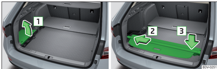
Fig. 135 Remove the left side cover / store roll-up cover
