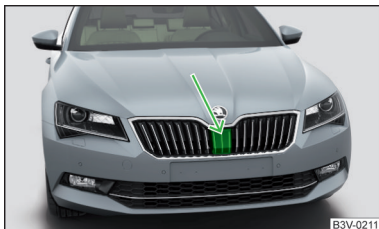
Fig. 174 Mounting location of the radar sensor
