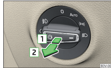
Fig. 57 Light switch – switch on front and rear fog lights
