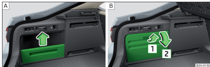
Fig. 138 Side shelf removal / open side pocket
