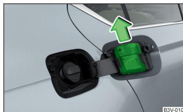
Fig. 223 Fuel filler flap: Remove ice scraper
