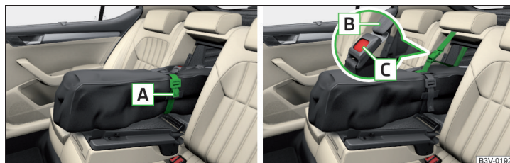
Fig. 109 Tighten ribbon / secure through-loading bag
