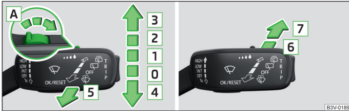
Fig. 69 Operation of wipers and washers: front / rear
