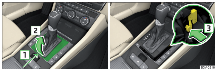
Fig. 263 Selector lever-emergency unlocking
