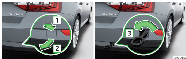
Fig. 253 Removing the cap / fitting the towing eye
