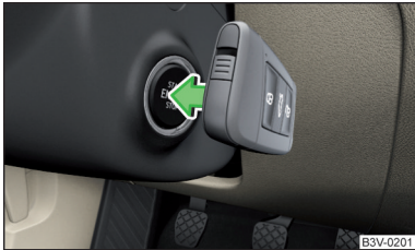
Fig. 163 Engine start - hold key on button
