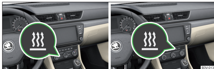
Fig. 159 Button for direct power on / off of the auxiliary heating (heating and ventilation) on the front panel of the Climatronic / manual air conditioning
