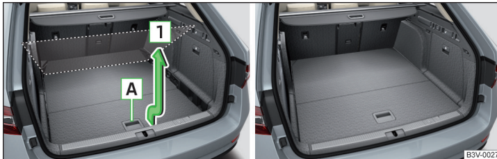
Fig. 145 Set variable loading floor to the upper position / variable loading floor in the upper position
