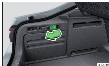
Fig. 79 Fold the backrest forward from the luggage compartment
