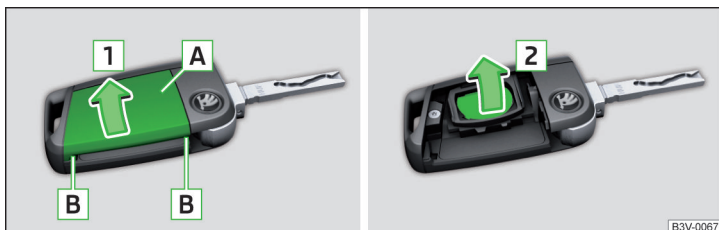
Fig. 254 Remote control key: Remove cover/take out battery
