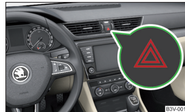
Fig. 58 Button for hazard warning light system
