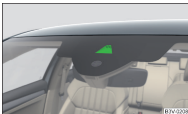
Fig. 217 Camera viewing range for traffic sign recognition
