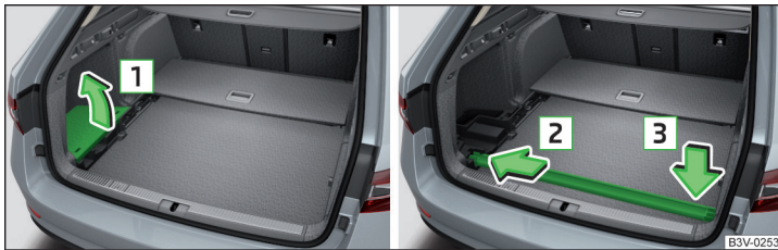
Fig. 137 Remove the left side cover / store multifunction tray
