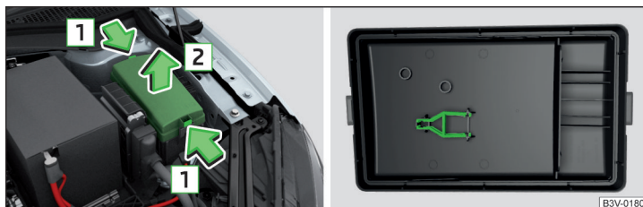
Fig. 269 Fuse box cover: remove cover / plastic clip for fuses
