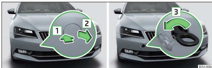
Fig. 252 Removing the cap / fitting the towing eye
