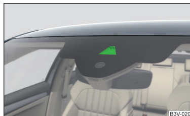
Fig. 211 Camera viewing window for Lane Assist
