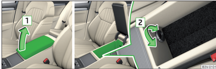
Fig. 98 Open tray / control air supply
