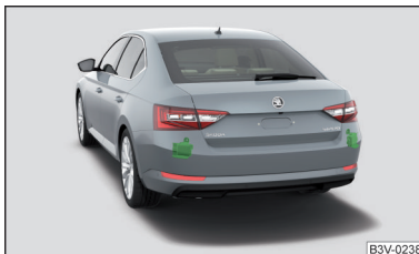
Fig. 214 Installation of radar sensors
