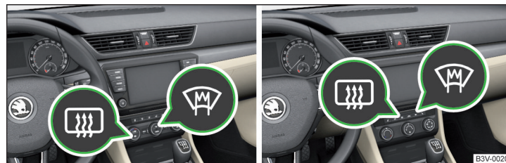
Fig. 65 Buttons for the front and rear window heater: Climatronic / manual air conditioning
