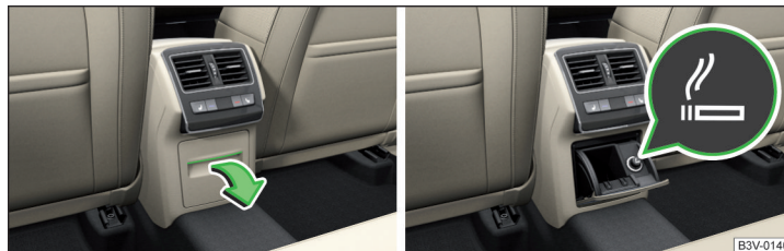
Fig. 118 Centre console at rear: Open storage compartment / cigarette lighter
