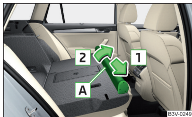
Fig. 151 Removing the net partition housing
