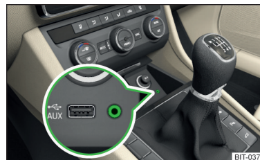
Fig. 111 Installation location if the AUX input
