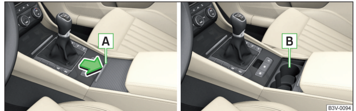
Fig. 94 Front centre console: Open cup holder / cup holder
