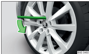
Fig. 245 Changing a wheel: Loosening the wheel bolts
