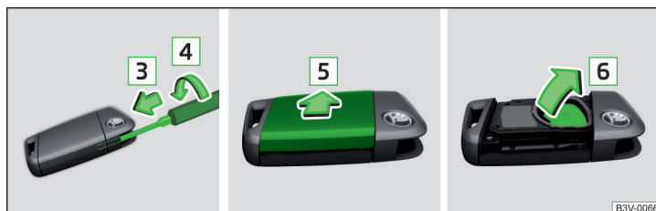
Fig. 256 Replacing the battery
