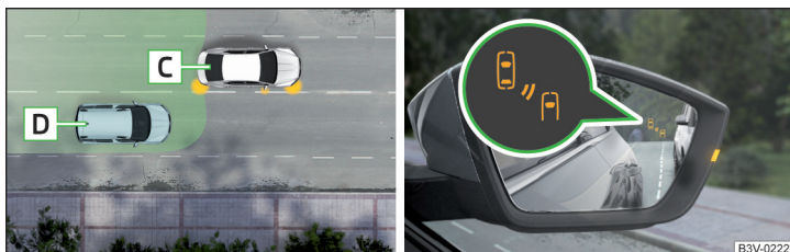
Fig. 216 Driving situation / indicator light in the right outside mirror indicates the driving situation
