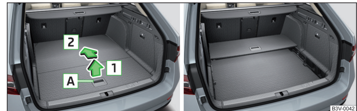
Fig. 147 Fold up variable loading floor / folded variable cargo floor in the upper position
