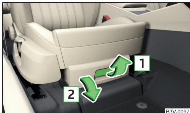
Fig. 102 Opening the storage compartment
