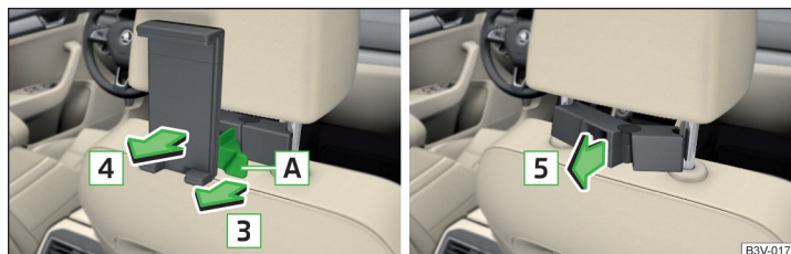
Fig. 123 Removing the holder/removing the adapter
