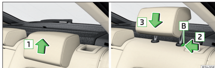
Fig. 83 Rear head restraint: moving it up / down
