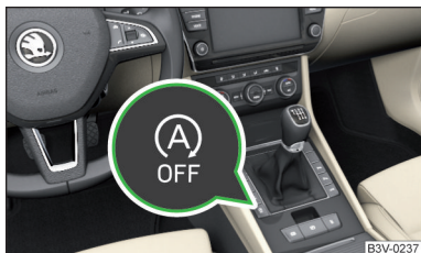
Fig. 165 Button for the START-STOP system
