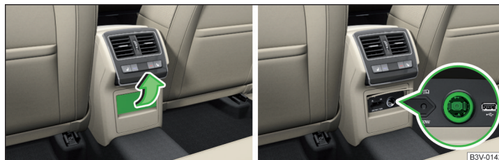
Fig. 113 Open the cover / 12 volt power outlet
