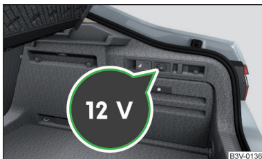
Fig. 115 Cover of the 12 volt power outlet
