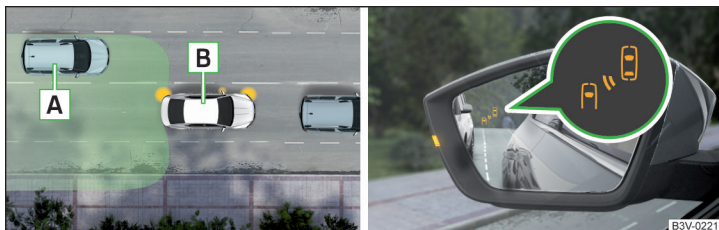
Fig. 215 Driving situation / indicator light in the left outside mirror indicates the driving situation
