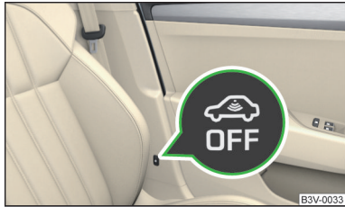
Fig. 43 Button for interior monitor and towing protection
