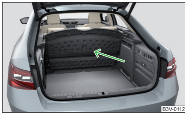
Fig. 133 Luggage compartment cover stowed behind the rear seats
