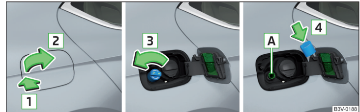
Fig. 226 Open fuel filler flap / unscrew tank cap / place the tank cap on the fuel filler flap
