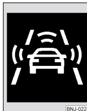
Fig. 208 Symbols in the instrument cluster: Warning or emergency braking at low speed
