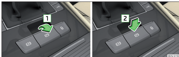
Fig. 167 Parking brake operation
