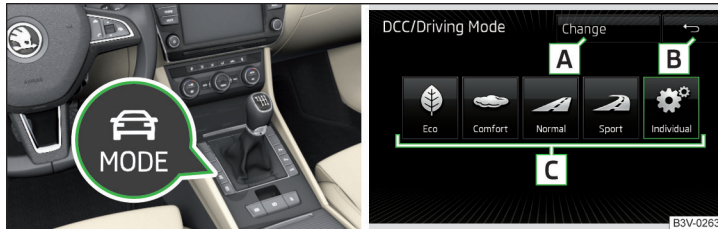
Fig. 210 Button for selecting the driving mode / Display in Infotainment display
