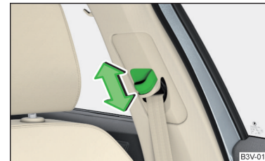
Fig. 6 Front seat: Seat belt height adjuster
