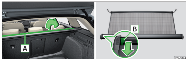
Fig. 149 Open part of the roll-up luggage compartment cover / release lever
