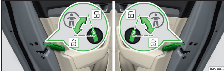
Fig. 42 Rear door: Child safety system switch on / off
