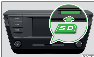
Fig. 201 Swing: Insert the SD card
