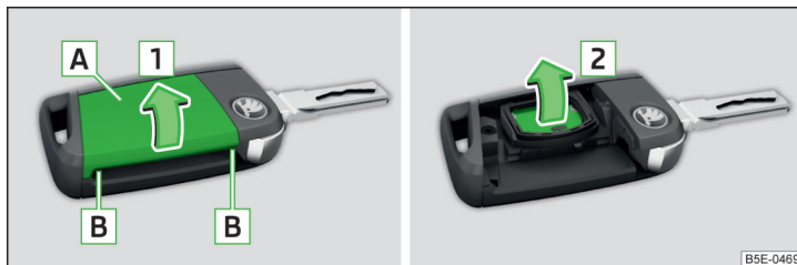
Fig. 342 Open the cover/remove the battery
