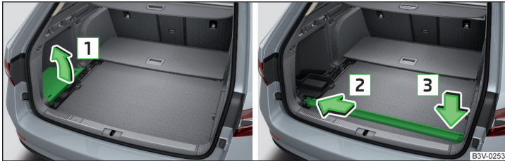
Fig. 156 Remove the left side cover / store multifunction tray
