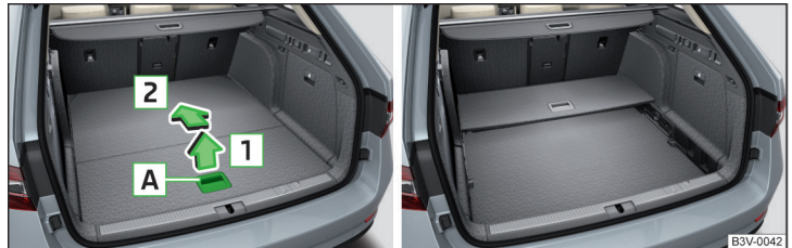
Fig. 161 Fold up variable loading floor / folded variable cargo floor in the upper position
