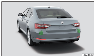
Fig. 275 Installation location of the radar sensors
