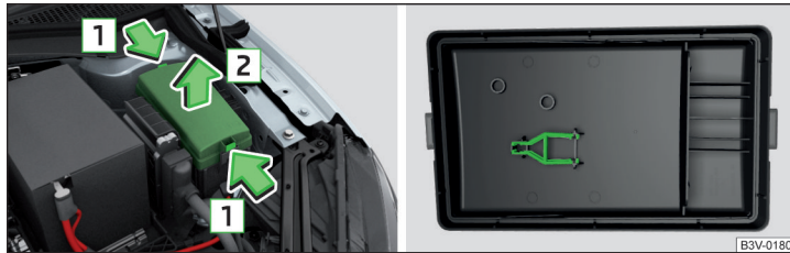
Fig. 360 Fuse box cover: Removing the cover / Plastic clip for fuses
