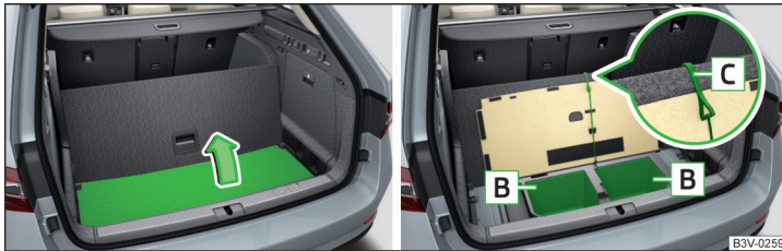
Fig. 154 Variant 2: Lifting floor covering/storage compartments
