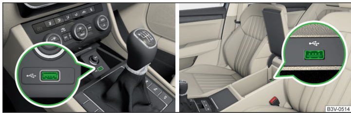
Fig. 110 Front USB input / USB input under the armrest
