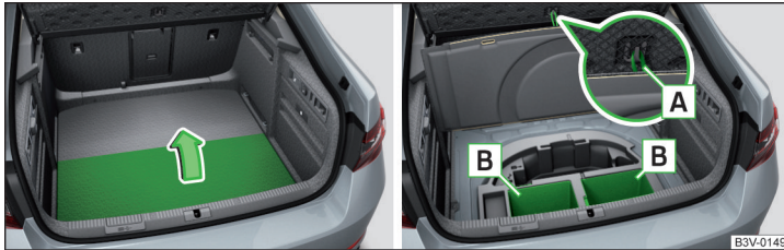
Fig. 153 Variant 1: Lifting floor covering/storage compartments
