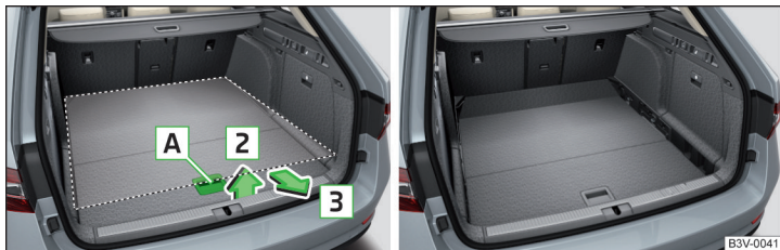
Fig. 160 Set variable loading floor to the lower position / variable loading floor in the lower position
