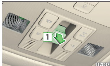
Fig. 63 Operation of the sliding/tilting roof
