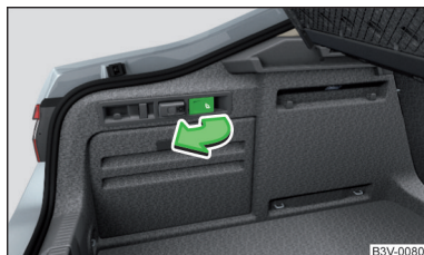
Fig. 94 Fold the backrest forward from the luggage compartment
