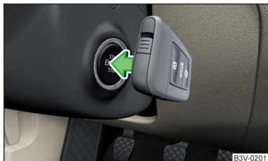
Fig. 256 Engine start - hold key on button
