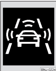
Fig. 302 Instrument cluster display: Advance warning or emergency braking at low speed
