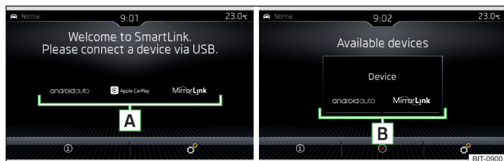
Fig. 218 Supported communication systems / Example of available communication systems of the connected external device
