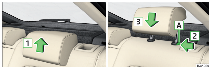
Fig. 97 Setting the height of the rear headrest
