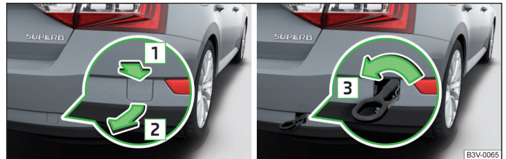
Fig. 341 Remove cap / install towing eye
