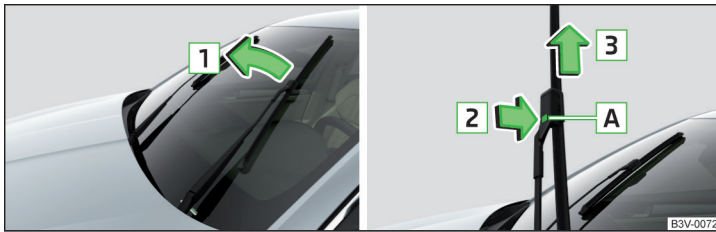
Fig. 353 Replace windscreen wiper blade
