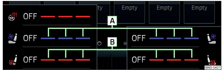
Fig. 103 Infotainment screen: Front seat heating and ventilation with maximum heating / ventilation level switched on
