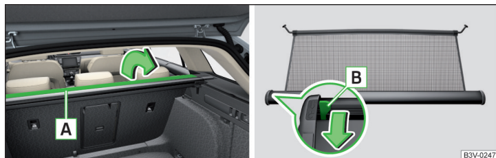
Fig. 163 Open part of the roll-up luggage compartment cover / release lever
