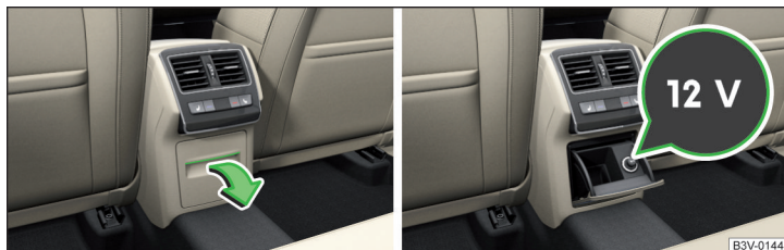
Fig. 130 Open storage compartment / cover of the 12 volt power outlet
