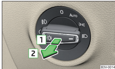
Fig. 69 Light switch – switch on front and rear fog lights
