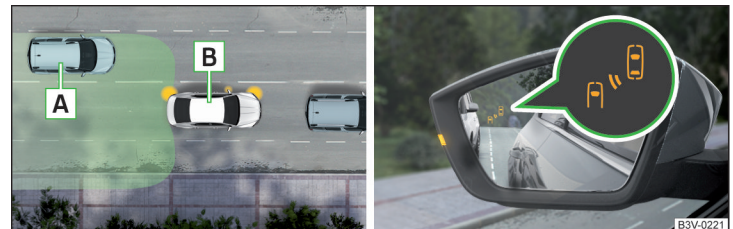
Fig. 277 Driving situation / indicator light in the left outside mirror indicates the driving situation
