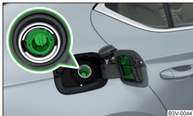
Fig. 315 Fuel filler tube on vehicles with diesel engines
