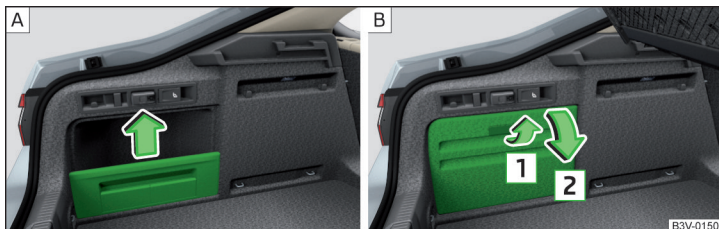
Fig. 150 Side shelf removal / open side pocket
