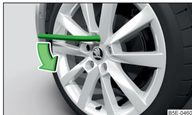
Fig. 334 Loosening the wheel bolts
