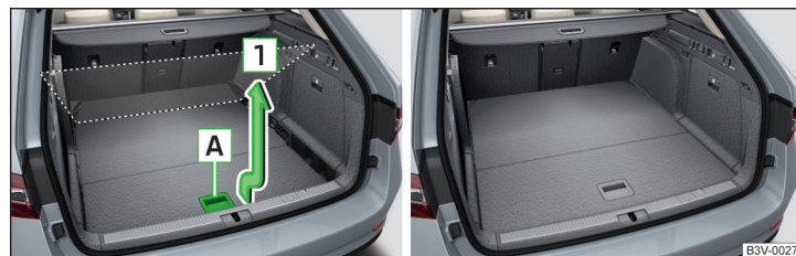
Fig. 159 Set variable loading floor to the upper position / variable loading floor in the upper position
