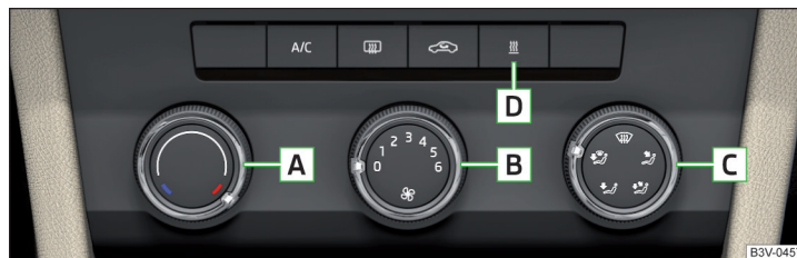
Fig. 167 Controls of the heating / air conditioning
