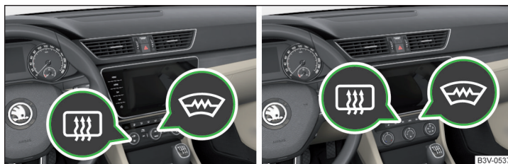
Fig. 77 Buttons for the front and rear window heater: Climatronic / manual air conditioning
