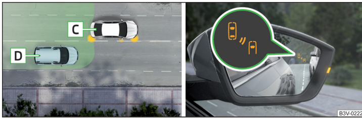
Fig. 278 Driving situation / indicator light in the right outside mirror indicates the driving situation
