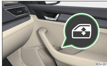
Fig. 61 Button of the window lifter on the passenger side
