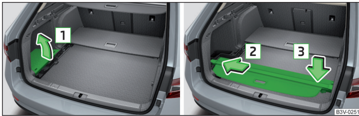
Fig. 149 Remove the left side cover / store roll-up cover
