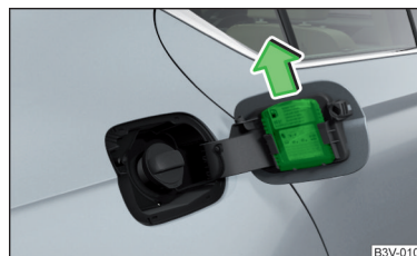
Fig. 312 Installation location of the ice scraper, removing the scraper
