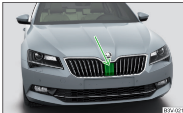
Fig. 268 Installation location of the radar sensor
