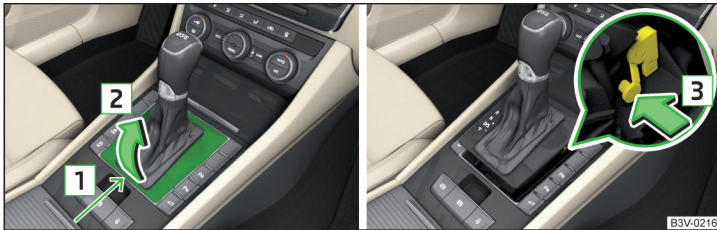
Fig. 351 Remove / release the selector lever
