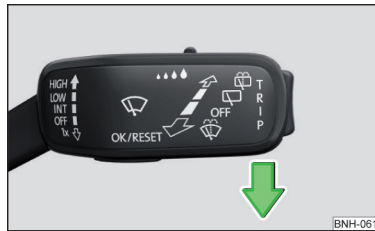
Fig. 352 Setting the service position for the wiper arms
