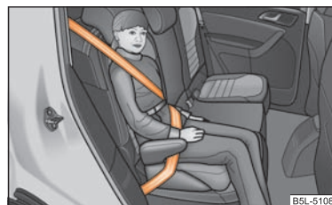
Fig. 147 Child seat in Group 3 installed on the rear seat facing the direction of travel
