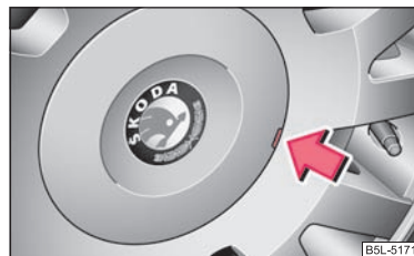
Fig. 180 Pulling off wheel trim cap on light alloy wheels
