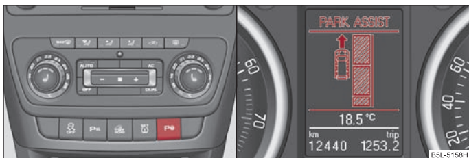
Fig. 114 Switching on the park assist/information display: Finding a suitable parking space
