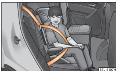
Fig. 146 Child seat in Group 2 installed on the rear seat facing the direction of travel
