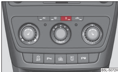
Fig. 106 Button for direct switching on/off of the auxiliary heating (auxiliary heating and ventilation) on the operating part of the air conditioning system
