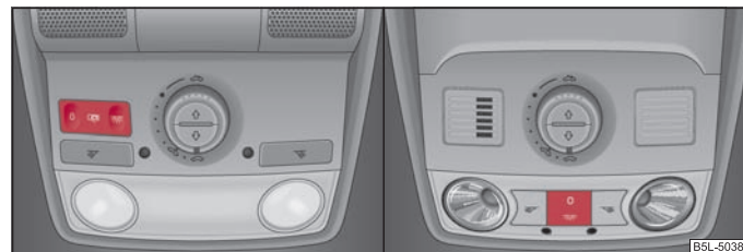
Fig. 44 Front vehicle interior lighting
