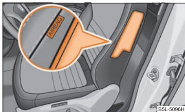
Fig. 138 Installation position of side airbag in driver seat
