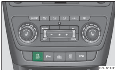
Fig. 150 ESP system: Switch for TCS
