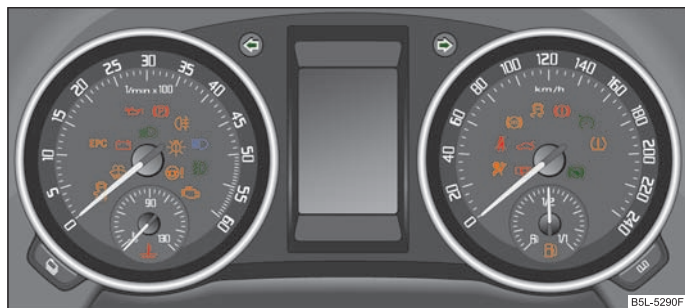
Fig. 21 Instrument cluster with warning lights
