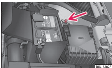
Fig. 186 Jump-starting on vehicles with the START-STOP system
