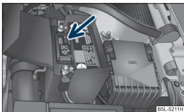
Fig. 171 The battery: Electrolyte level indicator
