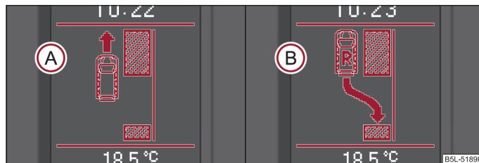
Fig. 115 Information display: the determined parking space with the information to drive on (A) and for engaging the reverse gear (B)
