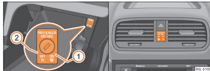
Fig. 142 Storage compartment: Switch for the front passenger airbag/indicator light for a switched off front seat passenger airbag
