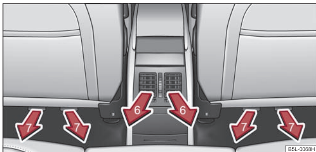
Fig. 102 Air vents at the rear
