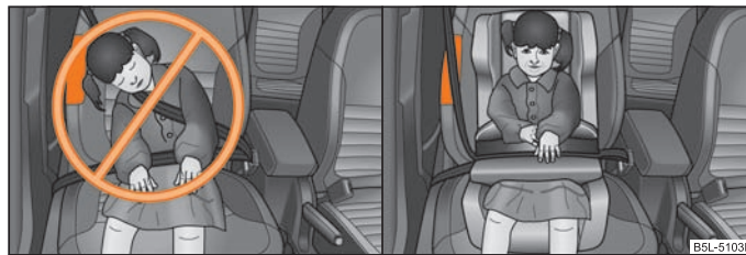
Fig. 143 Seated position of an unprotected child at risk from side airbag/Child properly protected by safety seat
