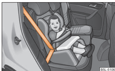
Fig. 145 Child seat with padded table in Group 1 installed on rear seat bench facing the direction of travel
