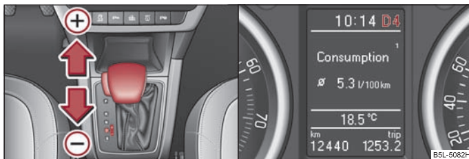
Fig. 120 Selector lever: manual shifting/information display: Manual shifting of gears
