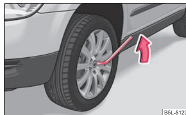
Fig. 181 Changing a wheel: Slackening wheel bolts
