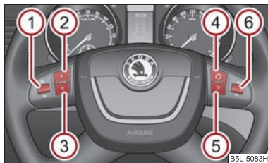
Fig. 122 Multifunction steering wheel: control buttons
