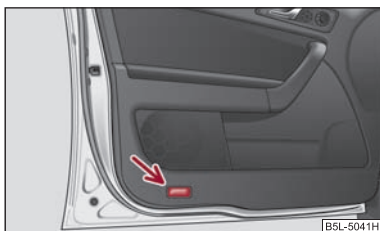
Fig. 47 Front door: Warning light
