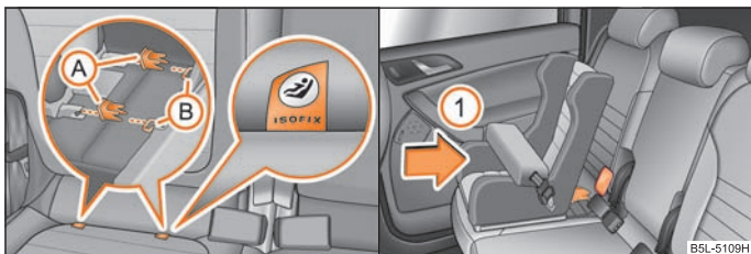
Fig. 148 Locking eyes (ISOFIX system)/the ISOFIX child seat is pushed into the mounting funnels
