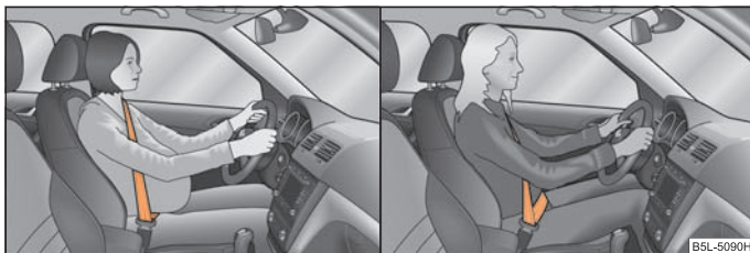
Fig. 131 Routing of belt webbing for an expectant mother/routing of belt webbing over the shoulders and the lap belt
