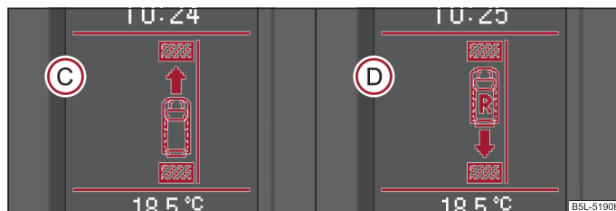
Fig. 116 Information display: Information for engaging the forward gear (C) or the reverse gear (D)
